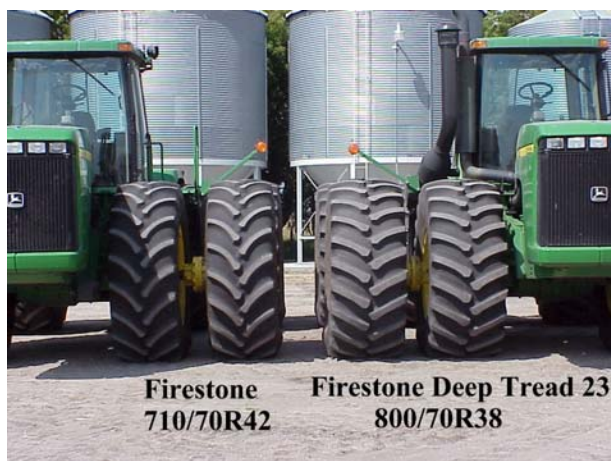
Figure 10. 710/70R42 tires versus 800/70R38 tires.
